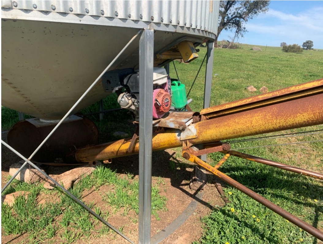
Photograph 17: Engine used to power auger. Photograph taken facing south west.
